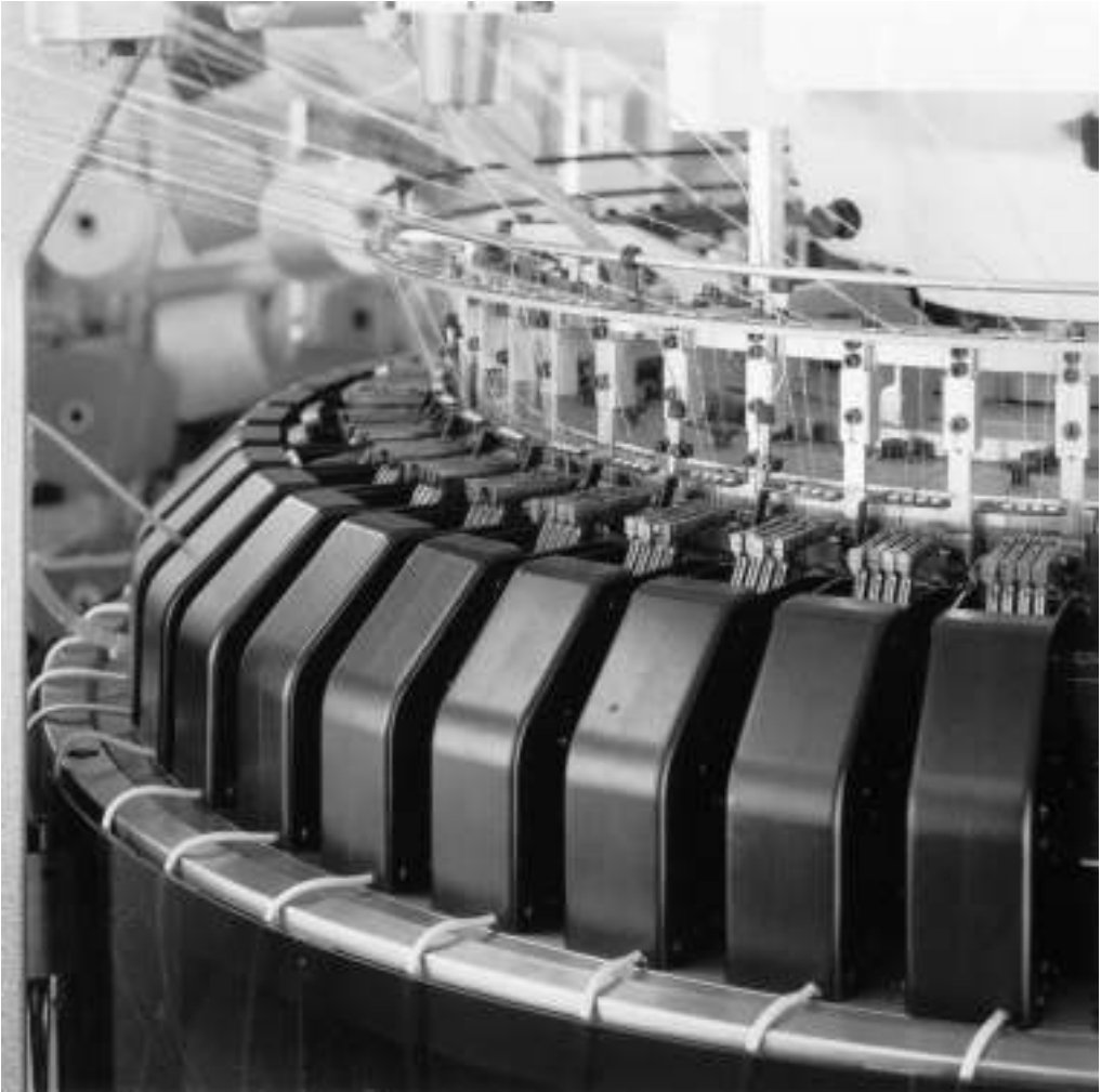
Fig. 11.11 Piezo-electronic rib jacquard machine with three-way selection and four-colour stripers [Terrot].
