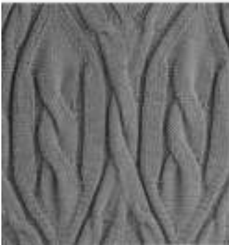
Widening with split-stitch (compound needle)
