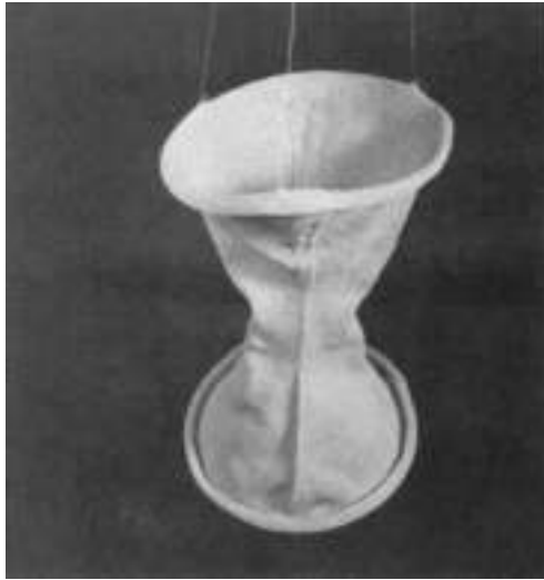
Fig. 30.7 Funnel-shaped tube connection in Kevlar [Stoll, from Knitting Technique , Vol. 13 (1991), 1, 123].
