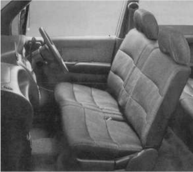
Fig. 30.5 Raschel-knitted spacer structure used for car seat covers of the Daihatsu Move 'Aero Down Custom' model. The front is formed as an openwork mesh structure and the back as a dense structure, so that the air circulates freely in the space between, and the driver and passengers are guaranteed an optimum microclimate [ Kettenwirk-Praxis (3/99), 40].
