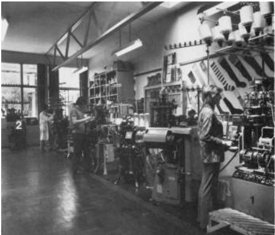
Fig. 8.4 Mechanically controlled hosiery machines. 1 = seamless hose machine; 2 = double cylinder half-hose machine.
