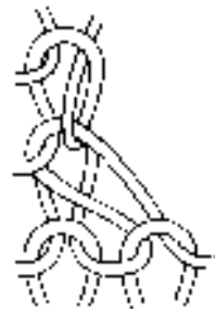
Fig. 6.8 Weft knitted loop transfer.
