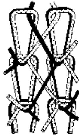
Fig. 6.11 Plating in warp knitting.
