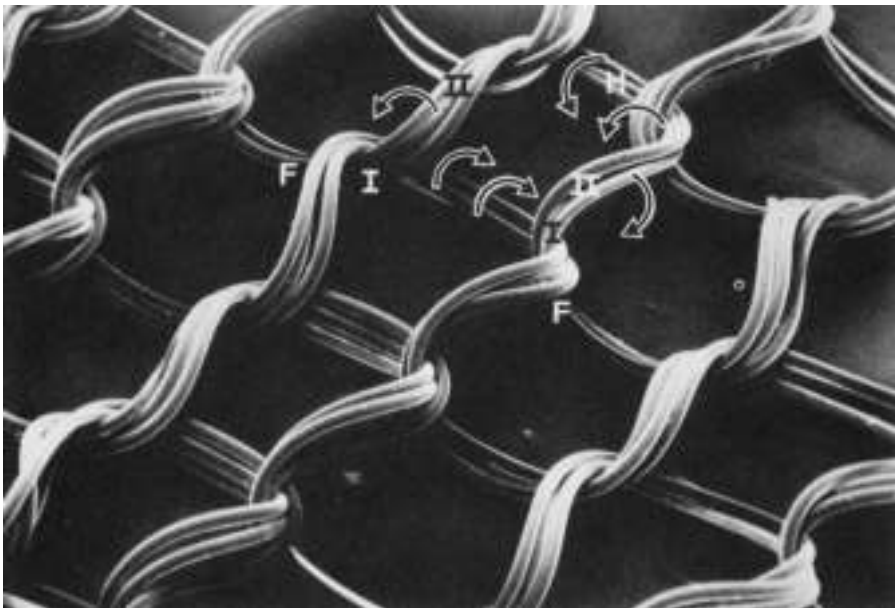
Fig. 7.3 The three-dimensional structure of plain weft knitting [Milliken AGILON] magnified \times 130 by a stereoscan electron microscope. The arrows indicate the direction in which the fabric will tend to curl if it is cut. [By permission of Knitting Times , official publication of NKSA USA].
