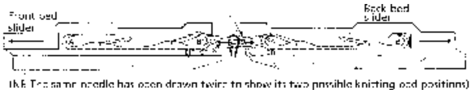
Fig. 7.17 Purl knitting using sliders.
