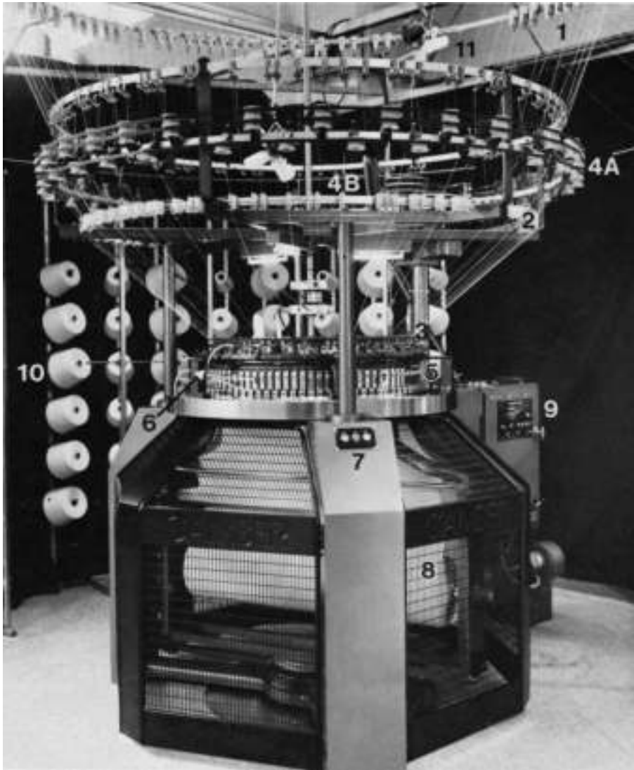
Fig. 13.12 The modern circular single jersey fabric machine.
