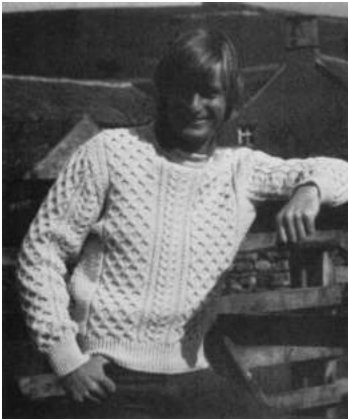
Fig. 18.8 Aran crew-neck pullover knitted by T W Kempton on a 5-gauge JDR flat machine from 2/6's worsted count woollen spun yarn [British Wool Marketing Board/Marks and Spencer].
