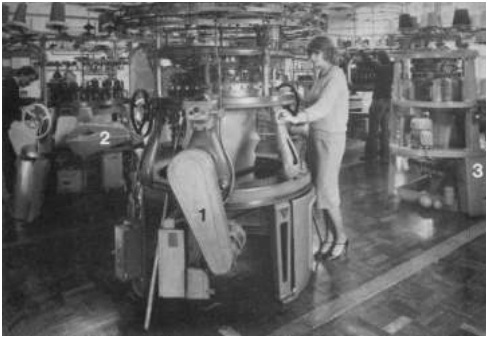
Fig. 8.3 Mechanically controlled circular knitting machines. 1 = plain cylinder and dial fabric machine; 2 = rib jacquard machine; 3 = double cylinder purl garment length machine.
